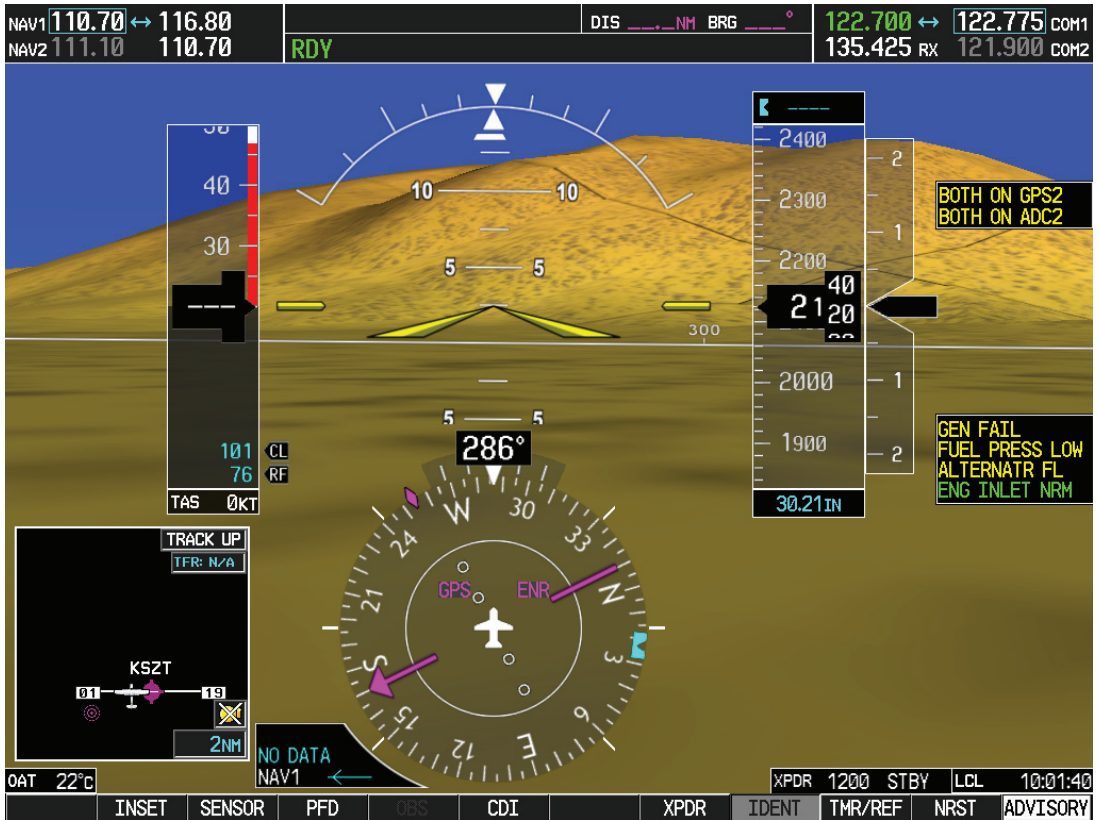
Figure 3-5 – No. 1 GPS/NAV Computer Failure (No. 1 PFD Shown, with Optional SVS System On)
