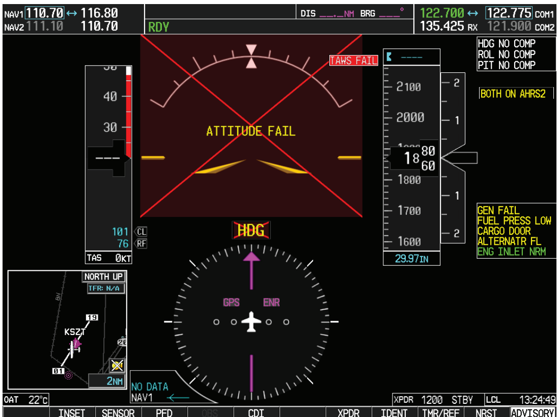
Figure 3-2 – Dual AHRS Failure (No. 1 PFD Shown)
