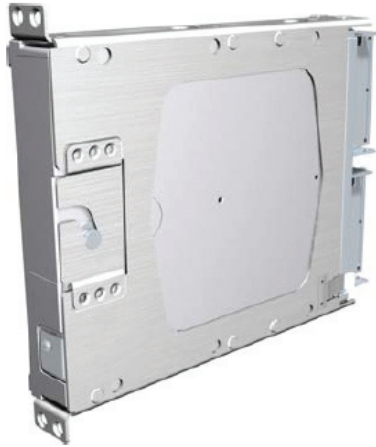
Figure 7-82 – GEA 71 Engine/Airframe Interface
