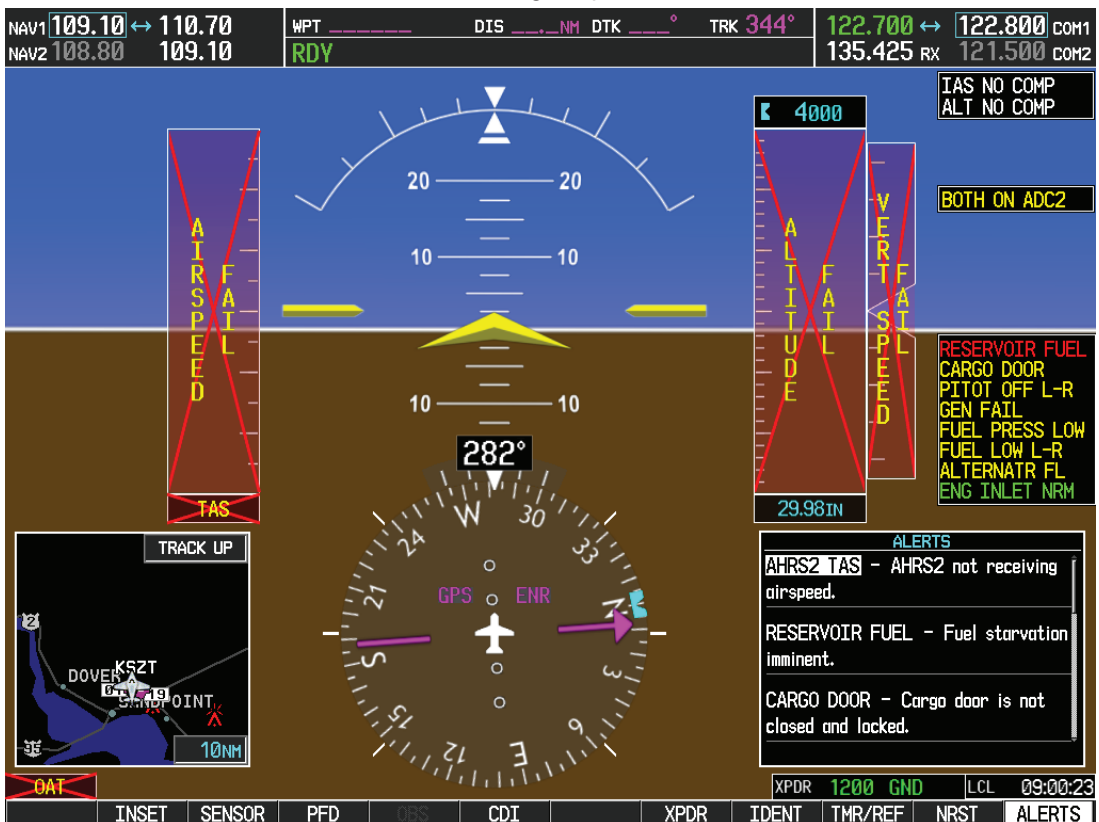
Figure 3-4 – Dual ADC Failure (No. 1 PFD Shown)
