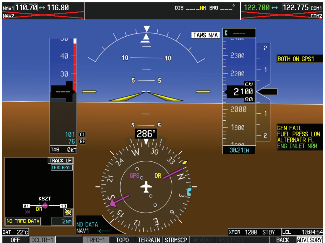
Figure 3-6 – No. 2 GPS/NAV Computer Failure (No. 1 PFD Shown)
