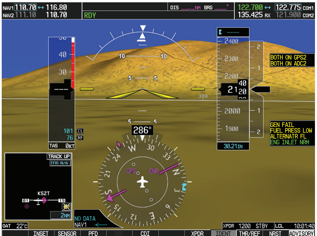
Figure 3-3 – No. 1 ADC Failure (No. 1 PFD Shown, with Optional SVS System On)
