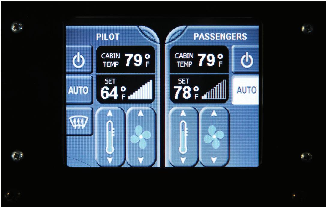
Figure 7-68 – ECS Touch Screen Display/Controller
