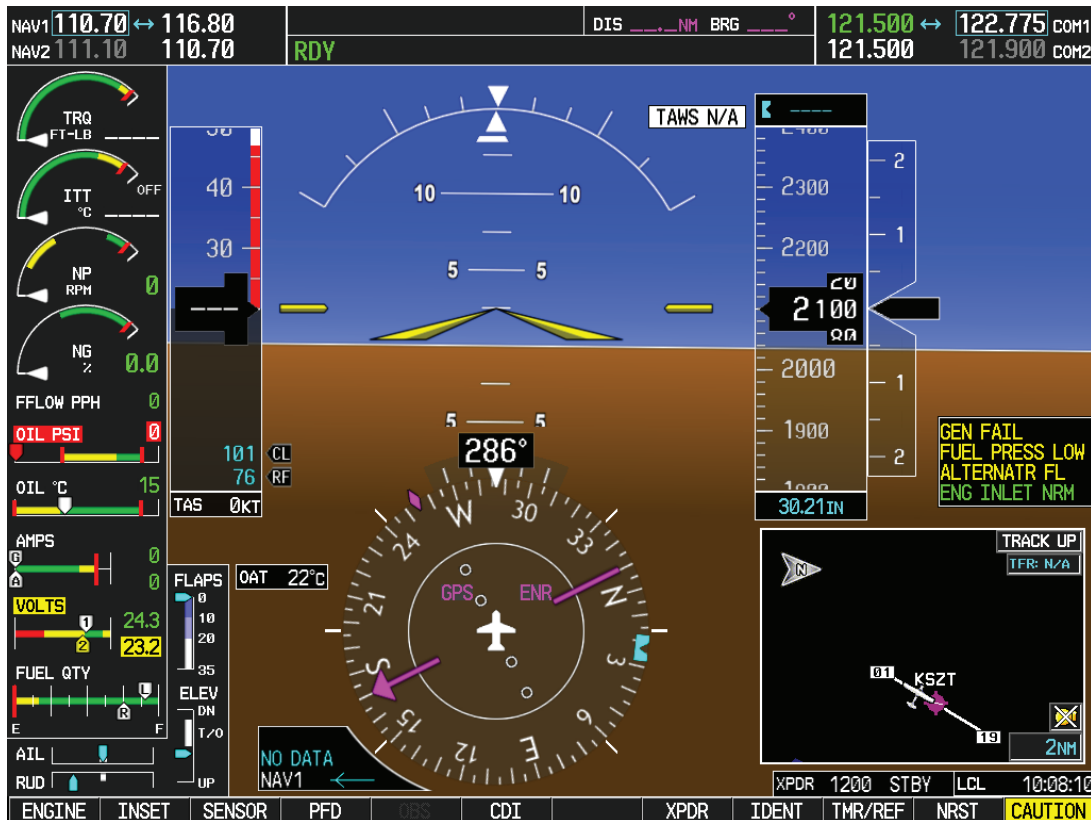
Figure 3-9 – Multi-Function Display Failure (PFD Shown)
